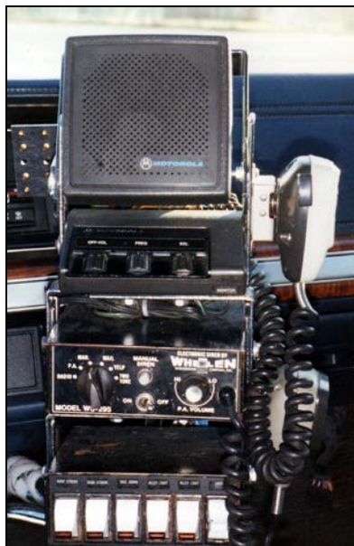
A “radio tree” set-up, first introduced in the 1991 Fords. The radio, public address, lights and siren controls were all within easy reach.
