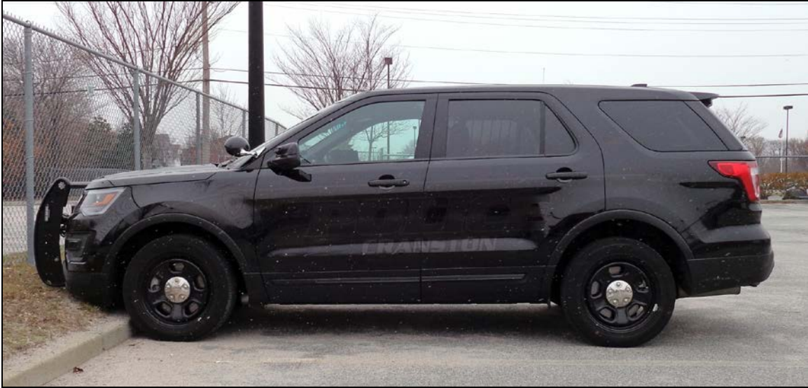
Some of the new patrol vehicles came equipped with “ghost graphics”; lettering that only shows up when illuminated by lights.
