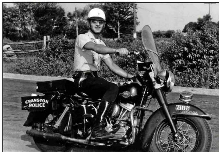
The motorcycle is a 1959-60 Harley-Davidson "Duo-Glide". It was equipped with a 55 horse-power, four-stroke, Panhead V-twin engine and could reach speeds up to 99 mph.
